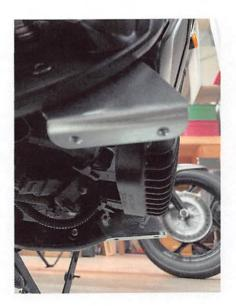
Now install the chin spoiler using the provided 1/4-20 buttonhead bolts and washers - applying Loctite 243 (BLUE) - to the threads of those 4 buttonhead bolts. DO NOT SKIP USING THE LOCTITE!!! Please feel free to email DOUG@DOUGZ.COM if you have any questions during installation.
