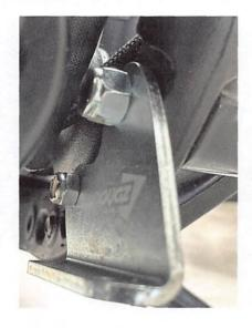
In the image to the left you see the chin mount fastened to the inside surface of the chassis, using the included 3/8-16 nylock nut, which is now threaded onto the longer Allen bolt from the previous step. Also, you see the 1/4-20 nylock nut threaded onto the Countersunk bolt mentioned in the previous step.
