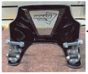
The chin spoiler is shipped with the mounting bolts in their proper location for reference during final assembly
